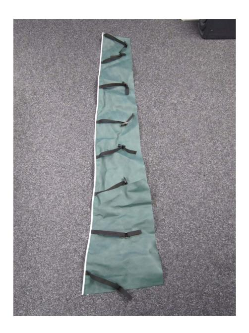
12. This strap strip is for the driver's side. The front of the caravan would be to the right of the picture. The grey strip on the left is the piping which would slide into the channel of the awning rail, and then each black strap extends towards the front
